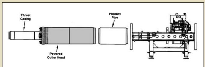
match the outside diameter of the larger pipe. The remaining soil around the previously installed 11-in. auger casings (Step 2) was taken into the PCH and discharged via the reception shaft by reversing the auger flight direction. The final product pipe was then installed directly behind the PCH. As each section of auger casing was removed from the reception shaft, a section of pipe was installed in the launch shaft. This step was completed when the PCH entered the reception shaft.
